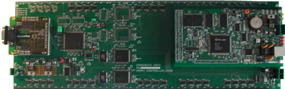
Local controller with 1 Gbps copper link and LAN interfaces
